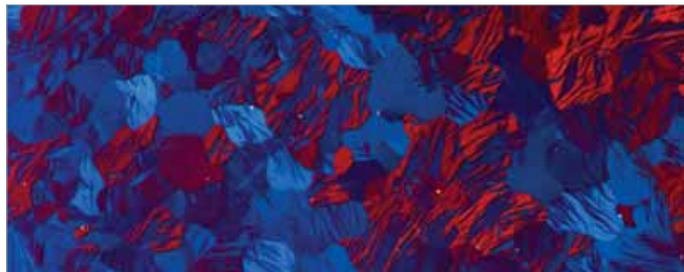
Pure magnesium, 100x, polarization
